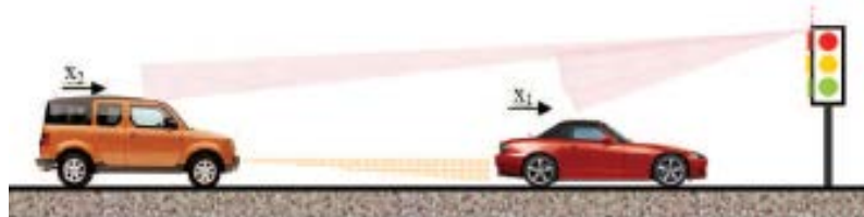
Figure 1: Schematic of telematics-based predictive cruise control
