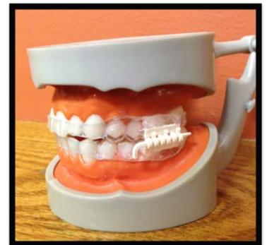
Figure 1: Customized Mandibulomaxillary Fracture Stabilization System with locking quick-release locking mechanism
