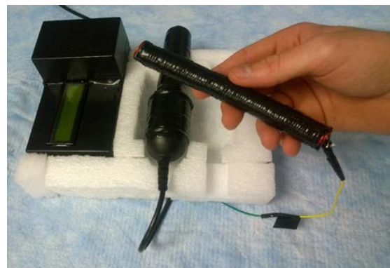
Figure 1: Functional titanium clip metal detector prototype. Wand will be used for handheld assistance in locating breast cancer.
